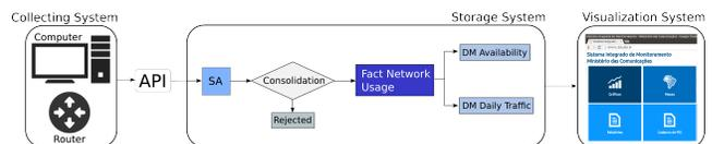
Figure 1: Data flow for SIMMC system.
