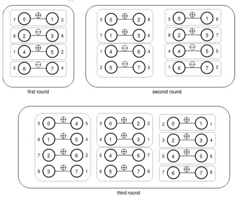
In the second round, when  $s \leftarrow 1$ , the exchange and comparison process is repeated considering two 2-dimensional hypercubes and then four 1-dimensional hypercubes. Finally, the last round of Algorithm 4 is equivalent to Algorithm 3 (see Figures 3 and 4). Note that in the last round, the ordering process starts with the bitonic sequence seq = (3, 6, 7, 8, 5, 4, 2, 1). At the end, the algorithm generates the sequence seq = (1, 2, 3, 4, 5, 6, 7, 8).
