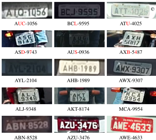
Fig. 11. Qualitative results obtained by the proposed ALPR system in the UFPR-ALPR dataset. The first two rows show examples of correctly detected and incorrectly recognized LPs, while the following rows show samples of LPs (from different categories) successfully recognized.
