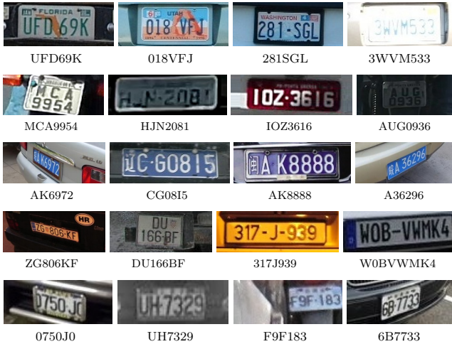
Fig. 12. Examples of LPs that were correctly recognized by the proposed ALPR system. From top to bottom: American, Brazilian, Chinese, European and Taiwanese LPs.
