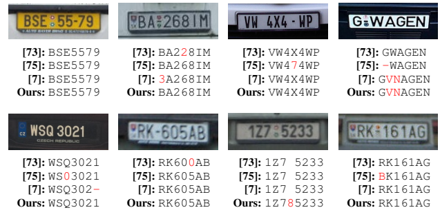
Fig. 19. Some qualitative results obtained on OpenALPR-EU [32] by Sighthound [73], OpenALPR [75], Silva & Jung [7], and the proposed system.
