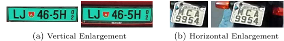
Fig. 3. Two illustrations of enlargement of the LPs detected in the previous stage. In this way, a single network is trained to recognize LPs of different layouts, regardless of their aspect ratios.
