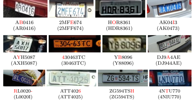
Fig. 13. Examples of LPs that were incorrectly recognized by the proposed ALPR system. The ground truth is shown in parentheses.
