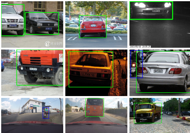
Fig. 7. Some vehicle detection results achieved in distinct datasets. Observe that vehicles of different types were correctly detected regardless of lighting conditions (daytime and nighttime), occlusion, camera distance, and other factors.
