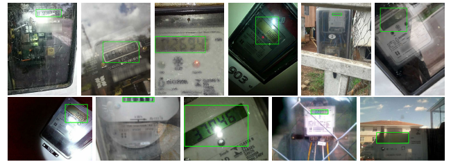
FIGURE 7. Representative samples of counters detected by the Fast-YOLOv4-SmallObj model – images taken under unconstrained conditions, e.g., with significant reflections, rotations, and scale variations.
