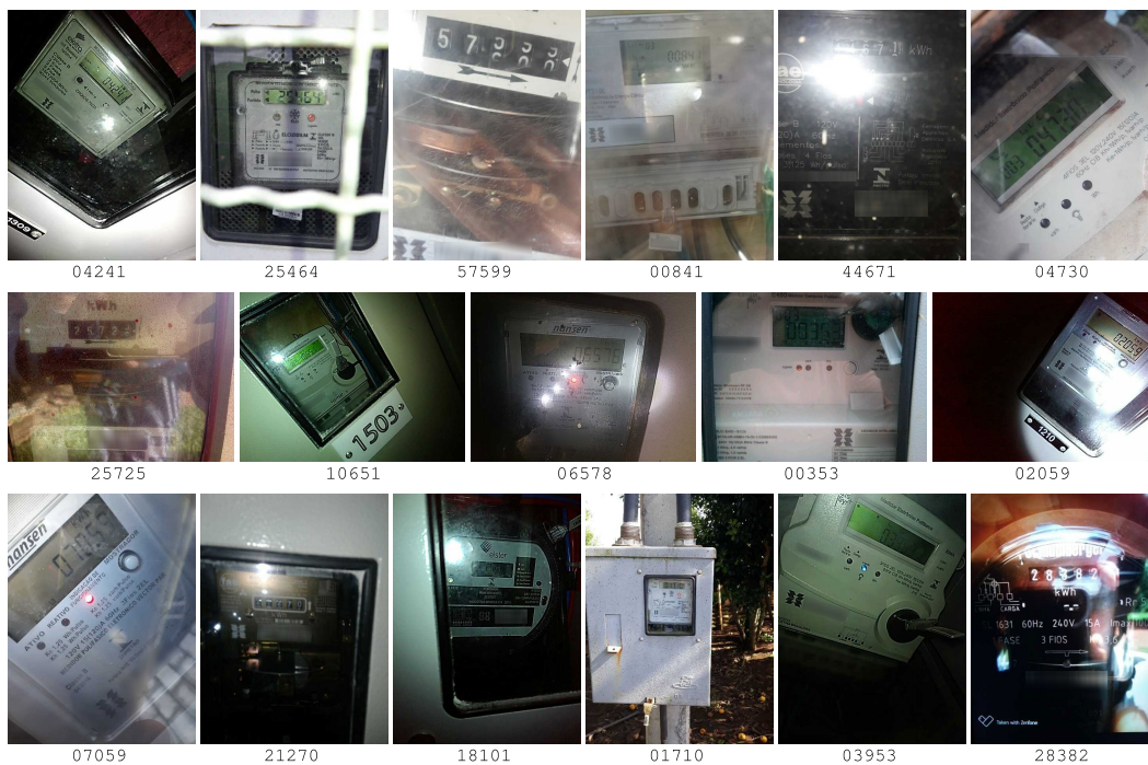
FIGURE 12. Examples of meter readings performed correctly by the proposed system. It is remarkable that it performed well in images of meters of different models and captured in unconstrained conditions (e.g., with various lighting conditions, reflections, shadows, scale variations, and considerable rotations).
