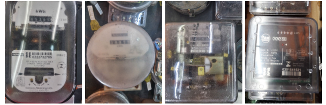
FIGURE 10. Some images from the UFPR-AMR dataset in which all evaluated methods failed to correctly perform the reading. In the first three images, there is dirt or water vapor on the meter glass, while in the fourth image the rightmost digit is labeled as ‘6’ and not ‘5’, contrary to the protocol normally adopted.
