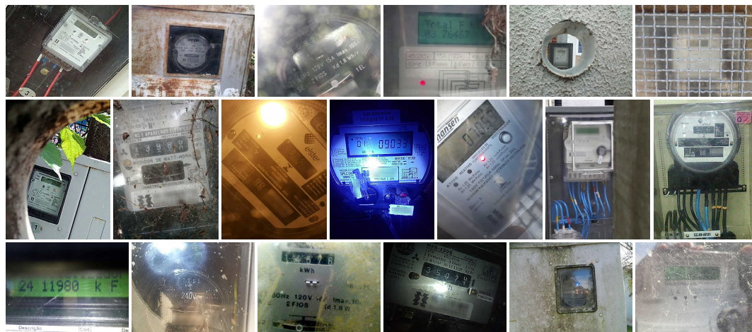
FIGURE 1. Some images extracted from the Copel-AMR dataset. Note that there are both electromechanical and electronic meters and that meters of different types/models often have different screen sizes and layouts. The last two images in each row are from faulty or illegible meters. As requested by Copel, the regions containing consumer identification were blurred on each image due to privacy constraints.
