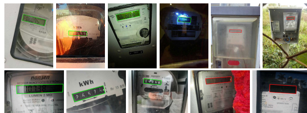
FIGURE 9. Some qualitative results achieved by CDCC-NET in corner detection and counter classification. For better visualization, we draw a polygon from the predicted corner positions. Counters classified as legible/operational are outlined in green while those classified as illegible/faulty are outlined in red.
