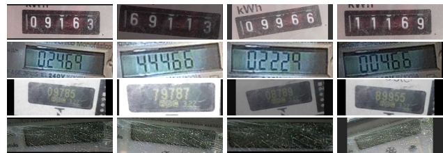
FIGURE 4. Some representative examples of the images generated by us for training CDCC-NET (and also Fast-OCR; see the next section). The images in the first column are the originals and the others were generated automatically.
