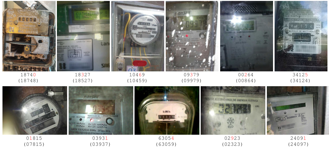
FIGURE 13. Examples of reading errors made by our system. The ground truth is shown in parentheses. Observe that most of the errors occurred in challenging cases, where even humans can make mistakes, as one digit becomes very similar to another due to rotating digits or artifacts in the counter region.
