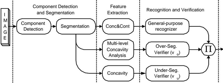
Fig. 5. Block diagram of the handwritten digit string recognition system.
