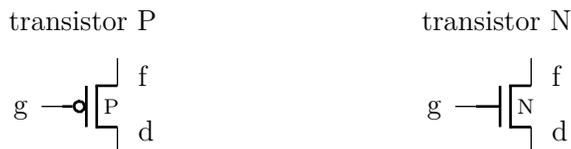
Figura 5.11: Transistores CMOS.
