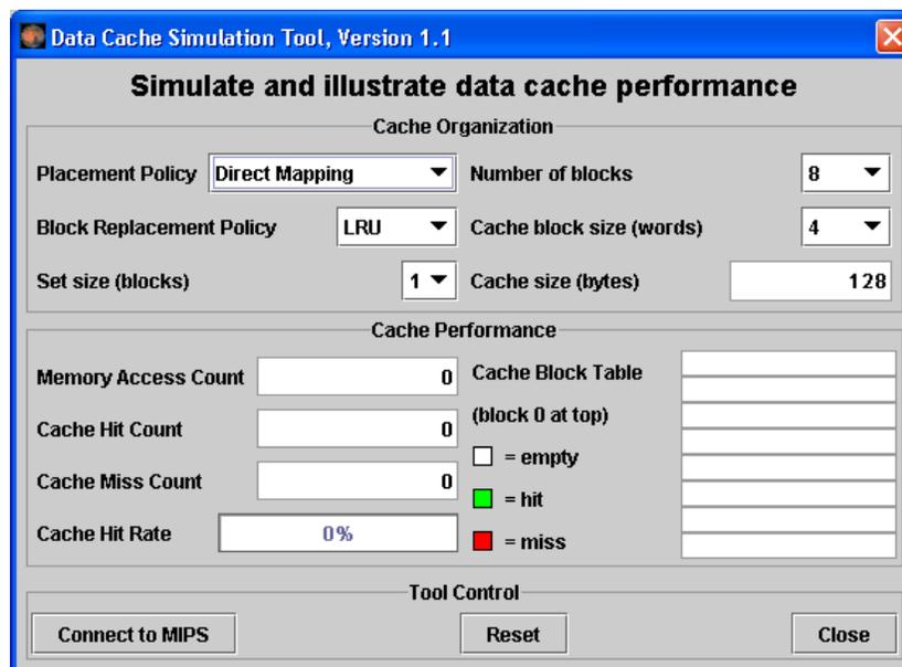
This is a MARS Tool that will simulate the use and performance of cache memory when the underlying MIPS program executes. Notice its three major sections:
