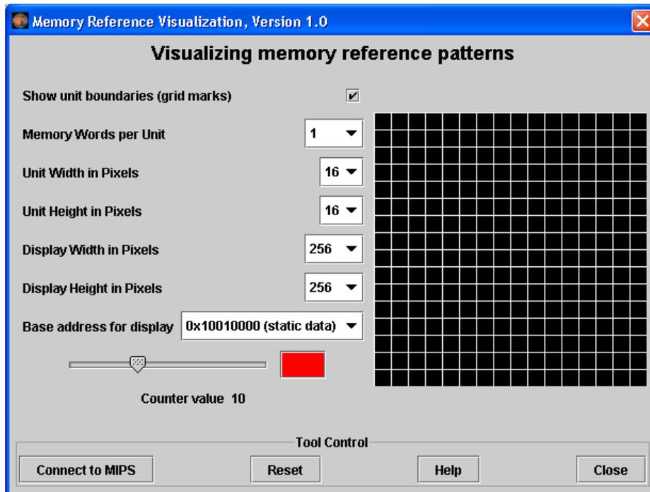
This tool will paint a grid unit each time the corresponding MIPS memory word is referenced. The base address, the first static data segment (.data directive) word, corresponds to the upper-left grid unit. Address correspondence continues in row-major order (left to right, then next row down).
