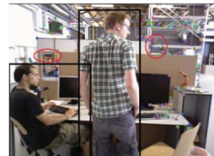
(c) Extract feature points after unifying gray values Fig.5 Feature extraction excluding dynamic object
