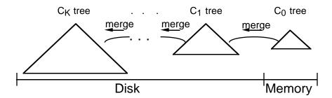
Figure 3.1. An LSM-tree of K+1 components
