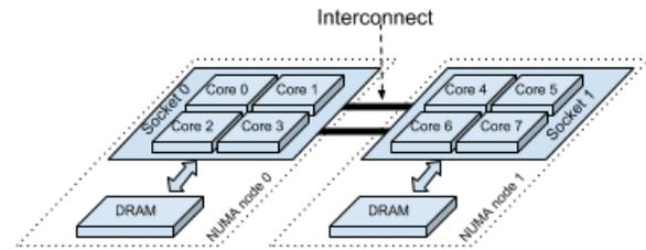
Figure 1: Schematic Diagram of the NUMA Architecture.
