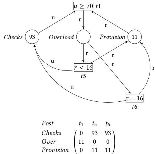
Figure 3: Tokenthrough transition in the Overload sub-net to allocate one core with  $u = 93\%$ ,  $r = 11$  out of  $rd = 16$  cores and  $th_{max} = 70\%$ .
