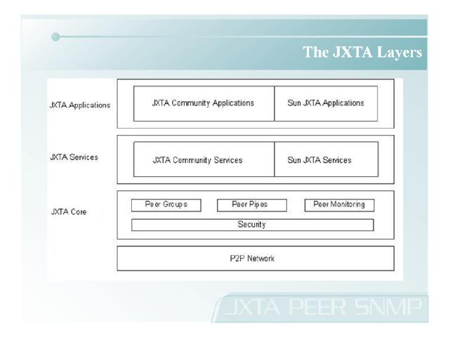
The JXTA platform is structured in three layers, as shown above. Each layer is based on the services of the lower layer, adding features and complexity. These layers are described in the following paragraphs.
