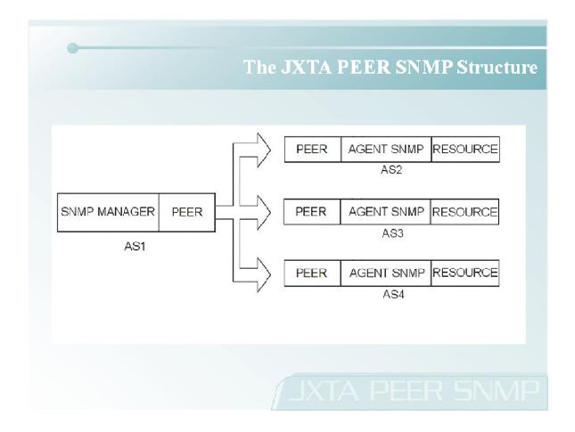
Using this system, a network administrator can manage resources in several AS's within a unified platform. The system is also secure, in the sense that it assures that only a JXTA PEER SNMP with permission (login and password) can have access to a group created by another JXTA PEER SNMP and be able to communicate with other peers in the group.
