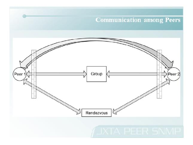
Each JXTA PEER SNMP needs, first of all, to connect with a rendezvous, the superpeer of the JXTA platform. After this initial connection is established, it is required to publish a peer group advertisement. The system performs this task automatically on demand. After a secure peer group is created, as described in the next section, each peer must join the group and, once inside the group, publish a pipe advertisement.
