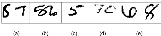
Fig. 18. Different classes of errors generated by the system: (a) Recognition errors, (b) ligature between two digits, (c) natural fragmentation, (d) fragmentation caused by noise, and (e) isolated digits classified as undersegmentation by v_u .
