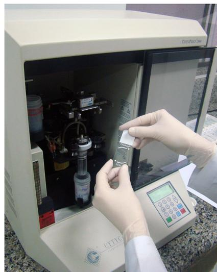
(b) Microscope slide being placed for processing in a Thinprep<sup>®</sup> 2000 processor. The procedure uses a liquid-based filtration process for slide preparation, whereby the sample is dispersed, randomized, filtered, and a representative sample is transferred to the slide. The automatic process guarantees the thin and uniform distribution of cells.
