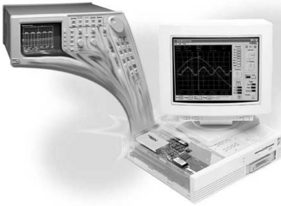
Figure 136-1 Virtual instrumentation: Replicating and enhancing traditional “vendor-defined” instruments with virtual “user-defined” instruments. (Courtesy of National Instruments.)
