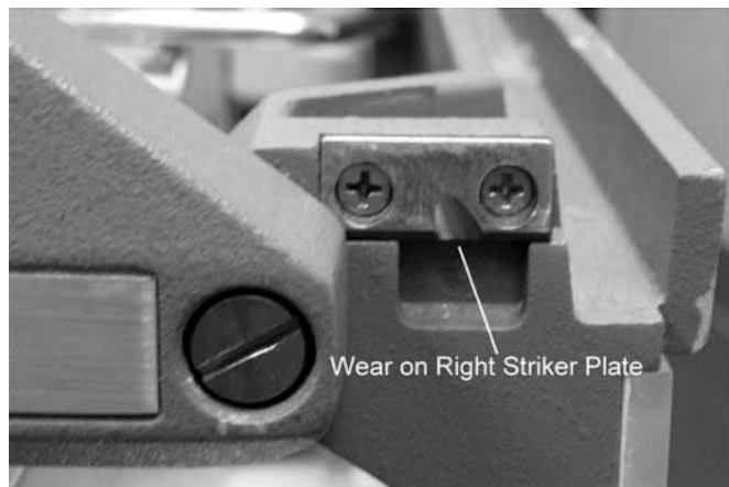
Figure 95-8 Incubator door latch striker plate showing wear to soft metal of plate. Such wear enabled an infant to open the door merely by the leaning on the door. Reproduced with permission from Shepherd (2003).
