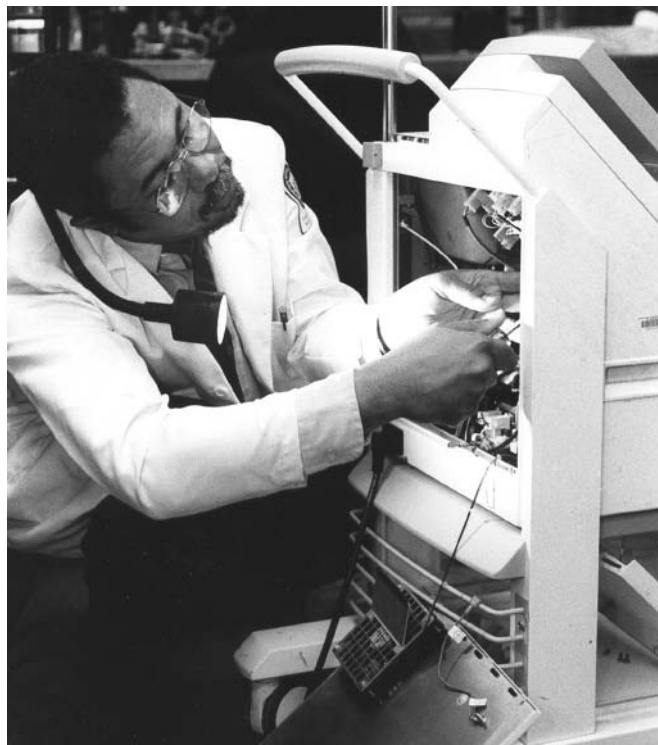
Figure 6-5 Preventive Maintenance. Senior biomedical engineer, Lenworth Howe, performing preventive maintenance on a cell saver. Preventive maintenance can be more involved than just performance of a functional and safety test. Problems uncovered must be rectified, and some instrumentation requires that components be replaced due to wear or number of hours of use.
