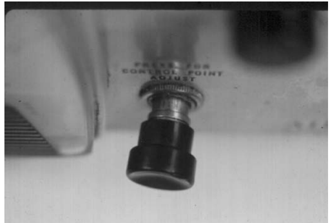
Figure 96-7 Front panel of an infant incubator, showing a bent knob.
