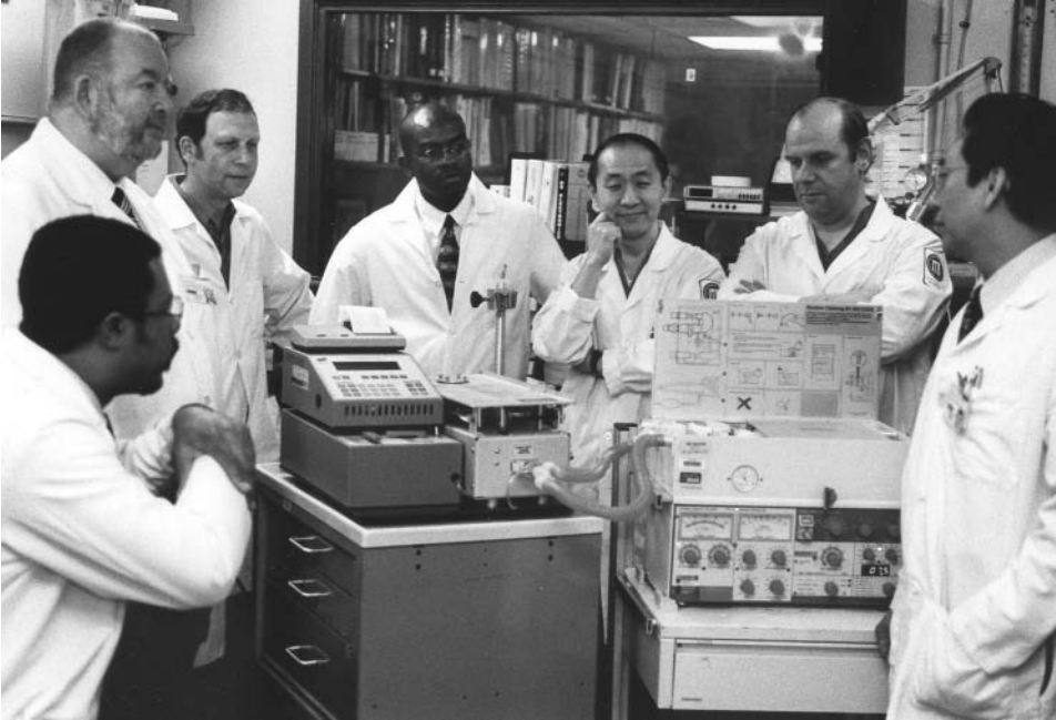
Figure 6-12 In-service Education. In-service education can be provided by manufacturers and vendors, as well as by clinical engineering staff. Here, Lab Supervisor, Luis Comejo, provides training to other clinical engineers in the use of an automated ventilator tester. Such devices reduce the number of individual test instruments required by integrating several test functions into one device, thus reducing service time leading to more rapid equipment turnaround. Such education also helps to satisfy JCAHO training requirements for clinical engineering staff.
