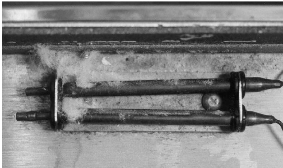
Figure 96-9 Lint and fluid accumulation on the temperature-control unit of an infant incubator.
