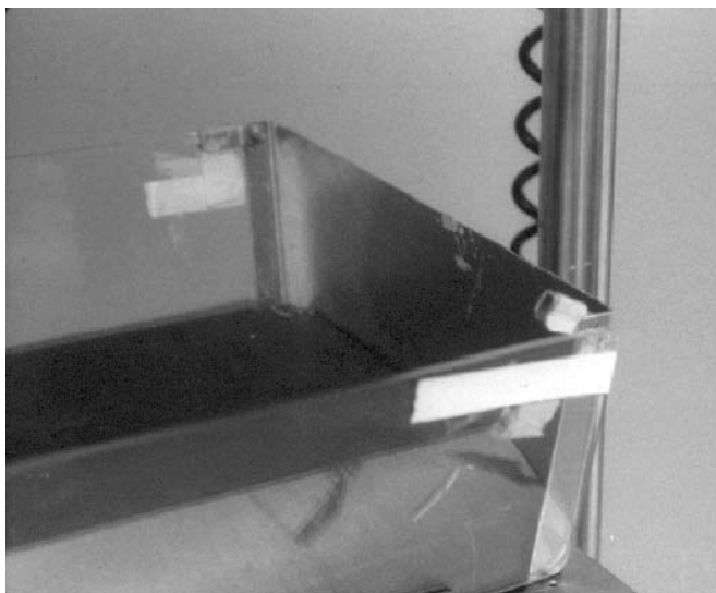
Figure 95-33 White tape fails to secure side panel.
