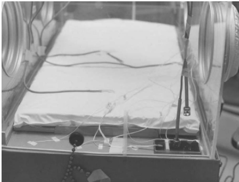
Figure 64-14 Surface temperature thermistors and an air temperature thermistor are shown affixed to surfaces and suspended above the air inlet vent of infant incubator in which infant suffered third-degree facial burns after contact with heated, humidified air at excessive temperatures. The hospital had not installed the plastic shield that the manufacturer made available as a retrofit.
