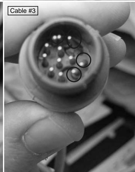
Figure 96-8 Bent pins on a connector, resulting from user error.
