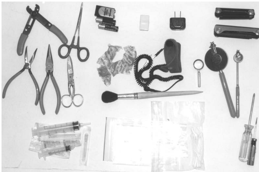
Figure 64-8 Contents of the lower tray. Upper row from left to right: wire strippers, forceps, batteries, adapter, electrical flasher, and Allen wrenches (metric and English). Middle row (l to r): curved tip pliers, needle nose pliers, scissors, Atomic Fireballs (candy to distract curious children during home investigations), camel hair brush, electrical grounding strap, 10X magnifier, inspection mirrors (large and small). Lower row from left to right: assorted syringes, plastic collection bags, cotton swabs, and screwdrivers (Philips head and small flathead).
