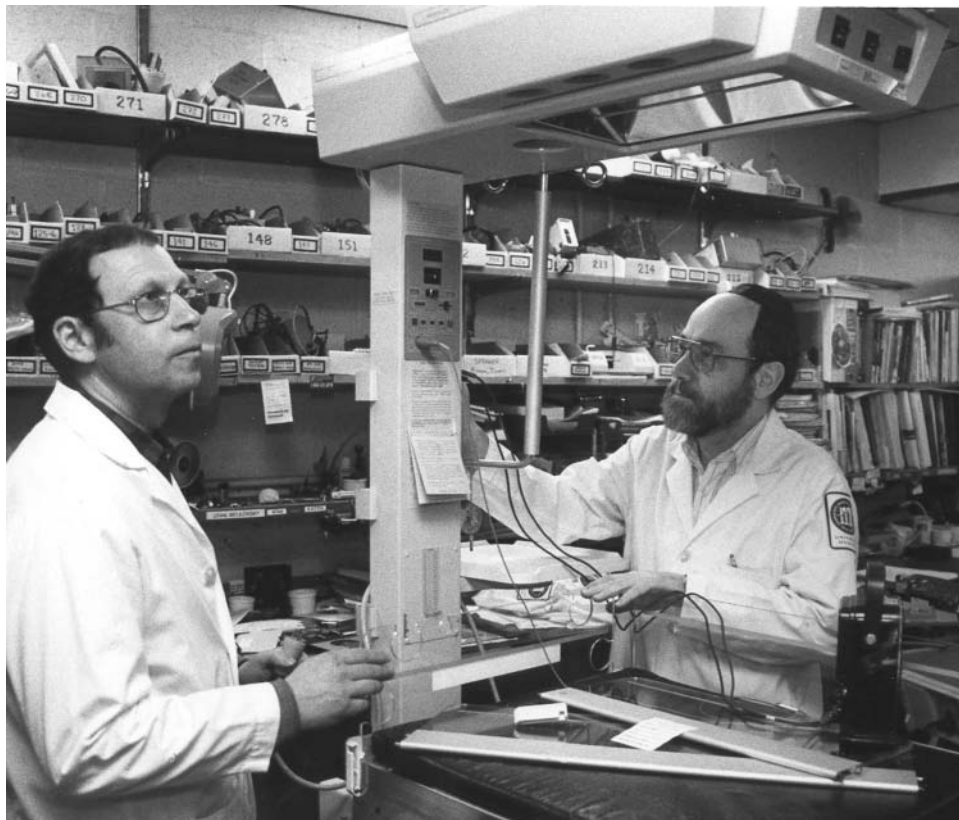
Figure 6-6 Repair. Senior biomedical engineers, Simon Gerecht and Michael Salts, utilize their extensive electronic troubleshooting skills during repair of an infant warmer to ensure that the thermostat controls are functioning properly.
