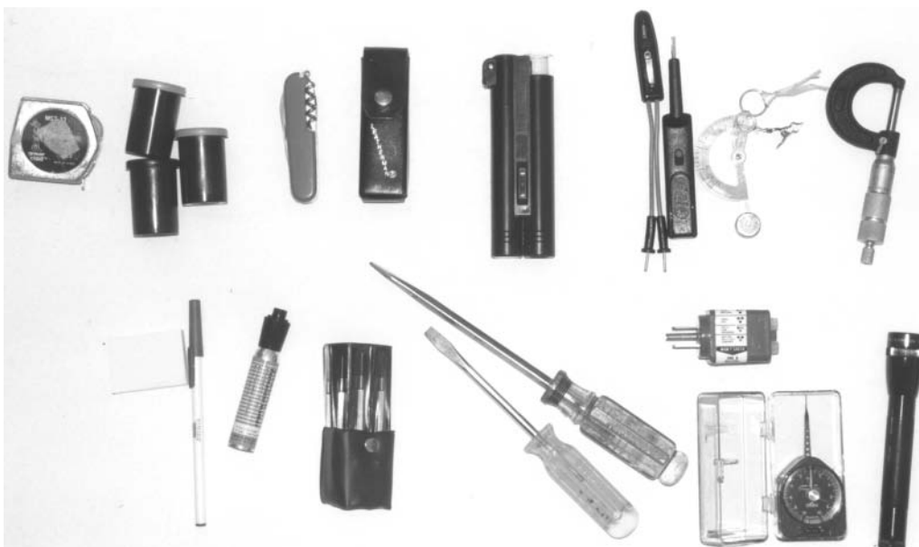
Figure 64-7 The contents of the upper tray. Upper row from left to right: tape measure, photographic film, Swiss army knife, Leatherman® tool, 30X illuminated magnifier, electrical circuit voltage tester and live circuit checker, letter scale (0-100 gm), micrometer. Lower row from left to right: Post-It notes, ball point pen, marking pen, jeweler's screwdrivers, screwdrivers (large and small flathead), receptacle tester, force gauge, flashlight.
