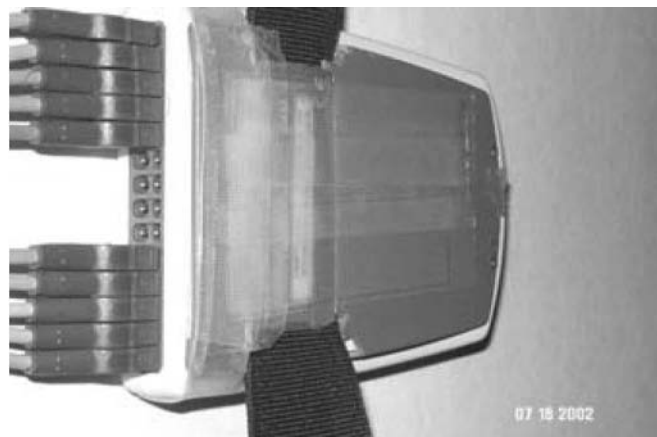
Figure 76-4 A 12-lead EKG interface secured with multiple layers of clear tape.
