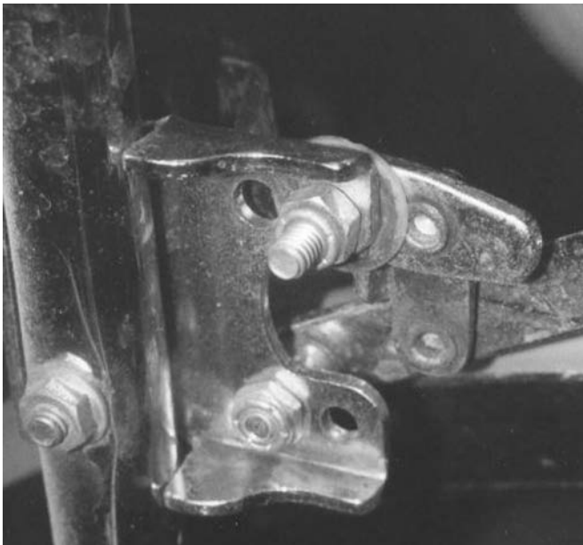
Figure 95-23 Brake mechanism of wheelchair.
