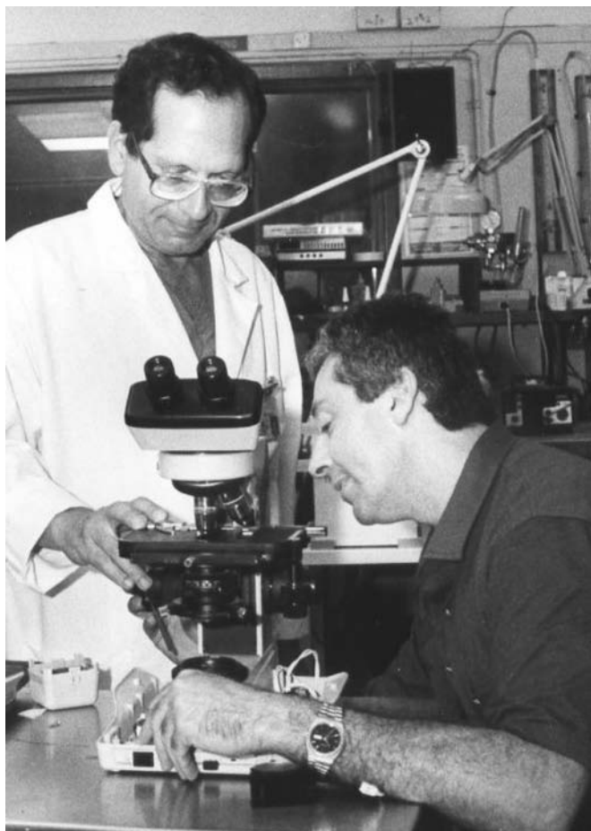
Figure 6-4 Acceptance Testing. Senior biomedical engineers, George Martin and Semyon Ulis, verifying correct operation of a newly purchased microscope to ensure that it is safe for use and that it performs according to manufacturer specifications, and rectifying any defects prior to its being released for clinical use. Payment is not authorized until the unit has successfully passed the acceptance-testing process.
